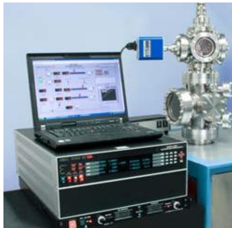
A typical lab set-up of a complete Kimball Physics system with power supplies, electron gun, and optional computer control system
