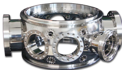
Figure 25. Custom 12" MCF™ Spherical Octagon vacuum chamber with 1) enlarged ports with increased conductance for better pumping efficiency and 2) offset port surfaces for specific design requirements.
