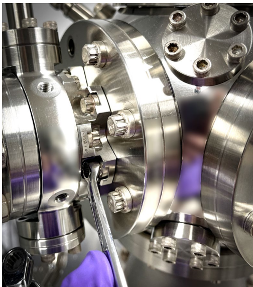
Figure 19. Silver plated bolts (#8-32, 1/4"-28 and 5/16"-24) used to secure flanges in a typical vacuum system. Allen hex heads with #8-32 bolts, and 12-point heads (1/4"-28, 5/16"-24) are present. Wrench in place to finish tightening 1/4"-28 bolt in limited space of a close coupler flange.
