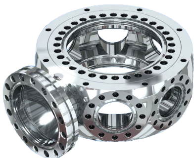
Figure 24. 6.0" MCF™ UHV Spherical Octagon with (2) 6.0" ports, (1) 4.5" high conductance welded, non-rotatable pumping port and additional (7) 2.75" ports. External mounting bracket capable with (8) threaded holes on each 6.0" flange face. Grabber grooves for internal mounting are present on all ports.
