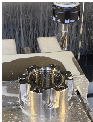
Figure 4. CNC fabrication in progress of flange features, with CF flange recess, knife edge, internal "grabber groove" channels being fabricated.
