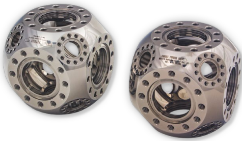
Figure 5. Spherical Cube Multi-CF™ Stainless Steel 316L (left) and Titanium Alloy (right) Spherical Cube UHV Vacuum Chambers with six (6) 2.75" (C) ports and eight (8) 1.33"(A) additional ports.
