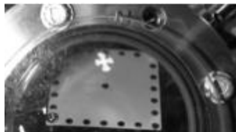
Maltese-cross shaped spot from an unfocused LaB 6 cathode seen on a custom phosphor screen inside the vacuum chamber.
