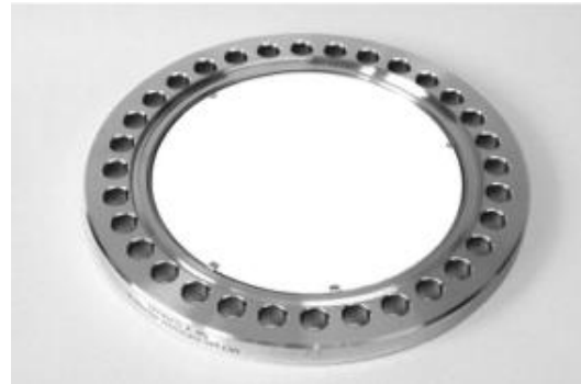
Thin Flange 6.00" CF with conductive glass backed phosphor screen mounted in the flange aperture. Small tabs secure the screen and conduct charge from the screen to the flange and then to ground.
