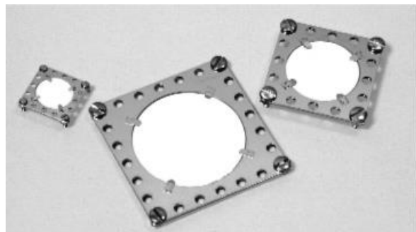
Examples of various sized Standard Phosphor Screens (0.7", 1.4" and 2.0" Edge length) with conductive glass (0.5", 1.0", 1.5" diameter) screens mounted in the central aperture of two adjacent square eV Part® plates. Tabs present to secure screens and conduct away charge.
