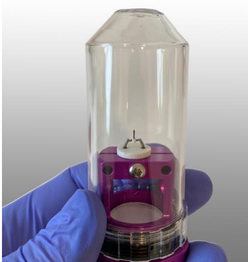
Figure 17. Cathode secured to base in transport container for safe storage and shipping.
