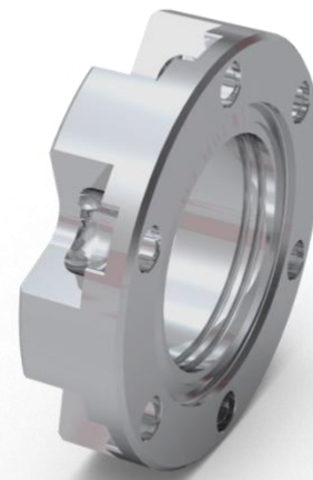
Tilt Adapter MCF275-TiltAdptr-C2-2Deg with two (2) 2.75" CF (C) sealing surfaces with base surface to right and 2-degree tilt surface behind and to the left. Note internal mounting channels (Grabber Grooves) associated with base flange.
