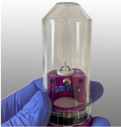
Example of Cathode Transport Container.
