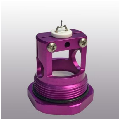
Example of Cathode with AEI base mounted in transport container.
