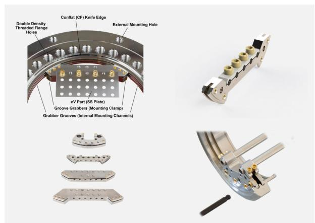
**Figure 7**. Upper left- Close up view of internal mounting "Grabber Groove" channels along the CF port internal bore, with a Groove Grabber mounting clamp engaging the mounting channels to securely support the internal apparatus. Other features of Kimball Physics CF ports shown including double density threaded flange holes, external mounting holes, and prototyping "eV" parts.
