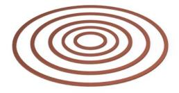
*Figure 20.* Nested copper gaskets for CF ports of 1.33", 2.5", 3.75, 4.5", 6.0", 8.0" and 10.0" are shown for size comparison of CF port apertures. The gasket thickness, 0.080" remains constant.
