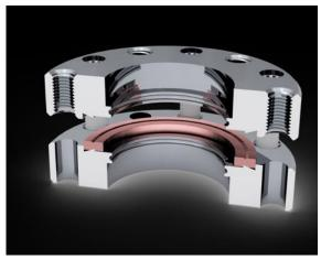
**Figure 6**. Schematic section view of CF flanges that were initially engaged and then separated to illustrate the sealing surfaces and the sealing groove created in the malleable copper gasket by the knife edges in the recess of the CF flanges.
