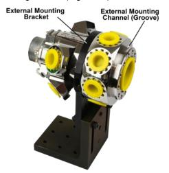
**Figure 10**. Spherical Octagon with bilateral mounting channels with External Mounting Bracket engaged. Temporary port covers are in place to protect CF surfaces including their knife-edges.
