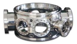
**Figure 25**. Custom 12" MCF<sup>TM</sup> Spherical Octagon vacuum chamber with 1) enlarged ports with increased conductance for better pumping efficiency and 2) offset port surfaces for specific design requirements.
