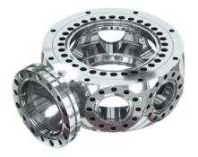
**Figure 24.** 6.0" MCF<sup>TM</sup> UHV Spherical Octagon with (2) 6.0" ports, (1) 4.5" high conductance welded, non-rotatable pumping port and additional (7) 2.75" ports. External mounting bracket capable with (8) threaded holes on each 6.0" flange face. Grabber grooves for internal mounting are present on all ports.
