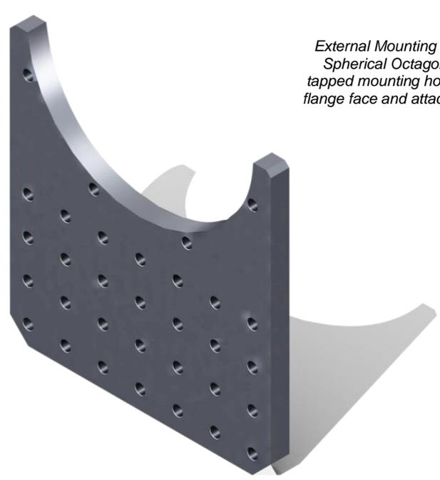
*External Mounting Bracket **MCF600-ExtBrkt-SM** for 6.0" Spherical Octagon MCF600-SphOct-F2C8. Mates via tapped mounting holes on the outer perimeter of 6.00" inch flange face and attaches to standard optical table hardware.*
