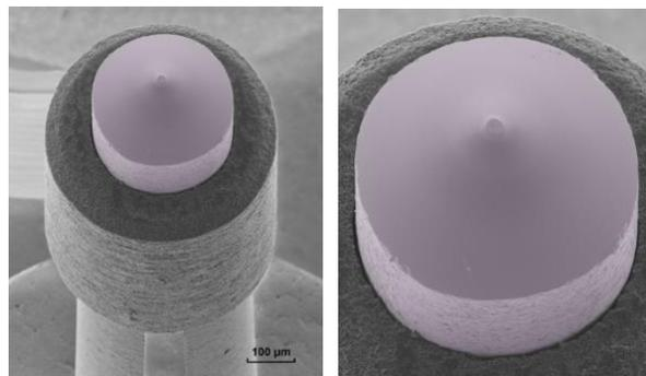
*SEM of LaB<sub>6</sub> single crystal cathode mounting with heating current path through precision-machined, single-piece carbon rod and <100> oriented LaB<sub>6</sub> crystal with 15 micron microflat at the apex of a truncated 90 degree cone geometry.*
