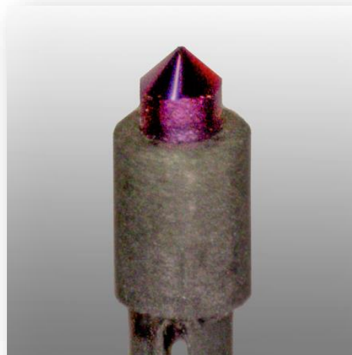
Cathode transporter with anodized aluminum base and sealable clear cover to protect the cathode during storage and transport. This example shows cathode ES-423E, a \text{LaB}_6 single crystal mounted on the end of a single piece of carbon heater rod, with a carbon ferrule to secure the \text{LaB}_6 .
