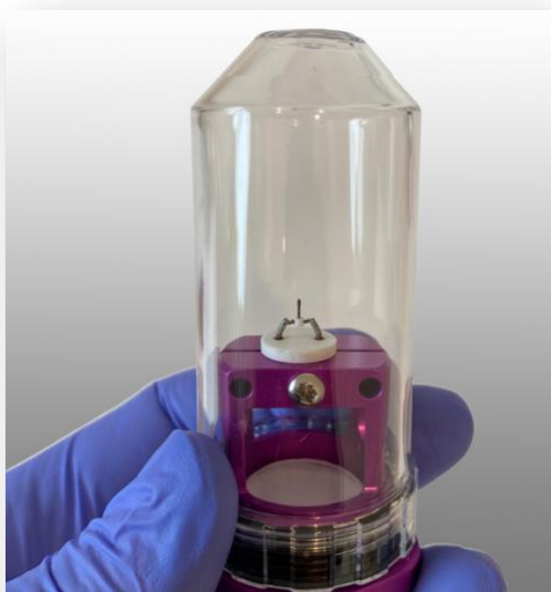
Cathode transporter with anodized aluminum base and sealable clear cover to protect the cathode during storage and transport. This example shows cathode ES-423E, a \text{LaB}_6 single crystal mounted on the end of a single piece of carbon heater rod, with a carbon ferrule to secure the \text{LaB}_6 .
