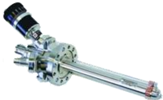
FRA-2X1-2 on a 2.75" CF Flange Multiplexer, with a rotary Faraday Cup
