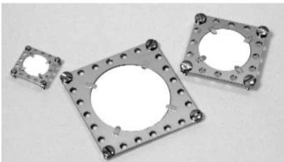
Examples of various sized Standard Phosphor Screens (0.7", 1.4" and 2.0" Edge length) with conductive glass (0.5", 1.0", 1.5" diameter) screens mounted in the central aperture of two adjacent square eV Part® plates. Tabs present to secure screens and conduct away charge.
