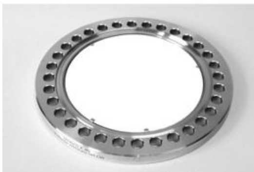
Thin Flange RHEED 6.00" CF with conductive glass backed phosphor screen mounted in the flange aperture. Small tabs secure the screen and conduct charge from the screen to the flange and then to ground.
