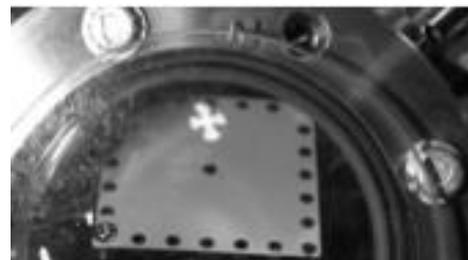
*Maltese-cross shaped spot from an unfocused LaB<sub>6</sub> cathode seen on a custom phosphor screen inside the vacuum chamber.*
