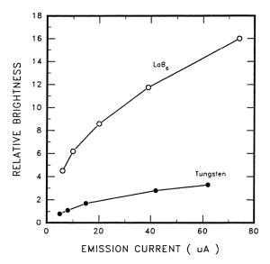
Figure 4. Relative brightness recorded from screen current versus total emission current for 5 Brightness settings with the emission at saturation. Data from Philips EM-420 TEM with  $LaB_6$  and tungsten cathodes.
