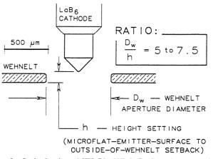
Figure 1. Scale drawing of KPI ES-423E LaB<sub>6</sub> Cathode set at height 125  $\mu$ m in a Wehnelt of 100  $\mu$ m thickness with an aperture diameter of 750  $\mu$ m. The ratio of  $D_w$  to h is 6, typical of that required for high brightness performance.
