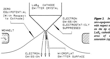
Figure 2 Intercept of the zero-equipotential (measured with respect to the cathode) on the tip of a truncated  $LaB_6$  cathode, defining the area of emission at saturation (optimum) bias.
