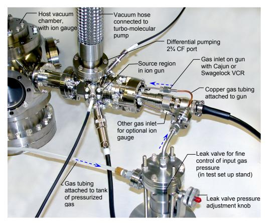
Fig. 4.8-1 A typical Ion Gun with Differential Pumping Port and optional Variable Leak Valve in a test setup
