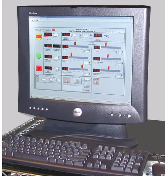
Fig. 4.1-5 Virtual Panel of a typical LabVIEW program for computer remote control and metering (Particular controls may vary with gun model)
