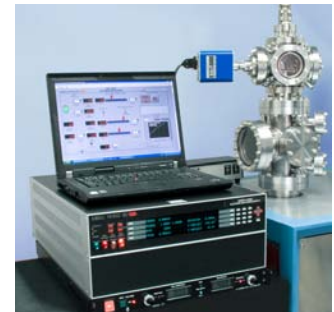
A typical lab set-up of a complete Kimball Physics system with power supplies, ion gun, and optional computer control system
