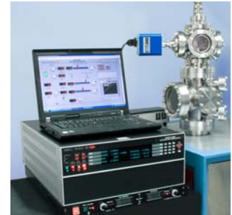
A typical lab set-up of a complete Kimball Physics system with power supplies, electron gun, and optional computer control system
