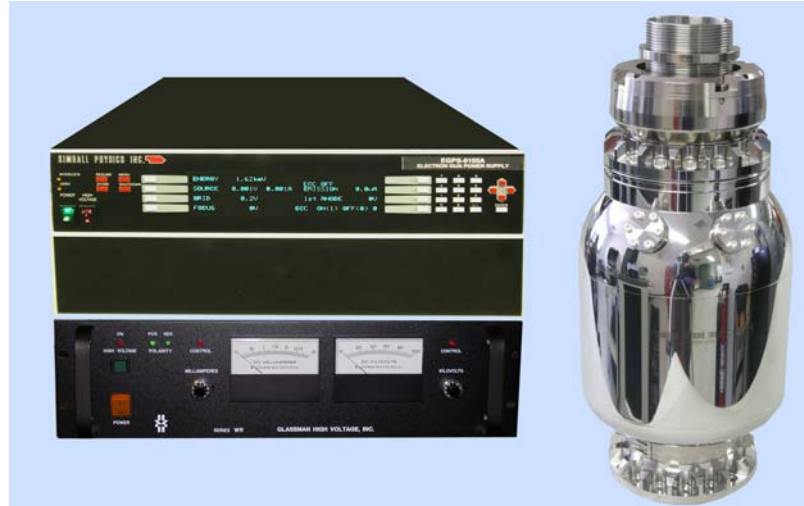
EGH-8105 Electron Gun System components - cables not shown
