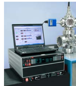
A typical lab set-up of a complete Kimball Physics high energy system with a focusable electron gun, power supplies and optional computer control system (details vary with gun model)
