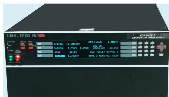
*EGPS-4104B Electron Gun Power Supply with FlexPanel controller*
