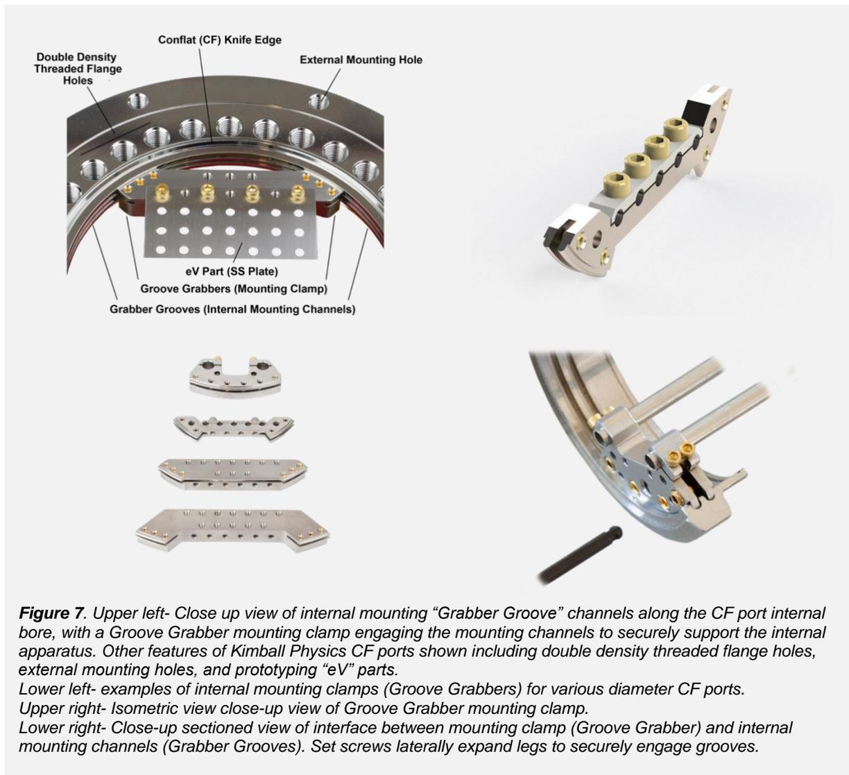
**Figure 7.** Upper left- Close up view of internal mounting “Grabber Groove” channels along the CF port internal bore, with a Groove Grabber mounting clamp engaging the mounting channels to securely support the internal apparatus. Other features of Kimball Physics CF ports shown including double density threaded flange holes, external mounting holes, and prototyping “eV” parts.
