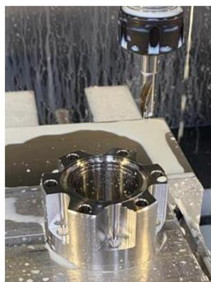
**Figure 4.** CNC fabrication in progress of flange features, with CF flange recess, knife edge, internal "grabber groove" channels being fabricated.
