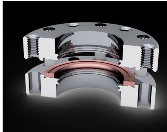
**Figure 6.** Schematic section view of CF flanges that were initially engaged and then separated to illustrate the sealing surfaces and the sealing groove created in the malleable copper gasket by the knife edges in the recess of the CF flanges.
