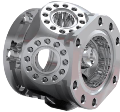
Flange Multiplexer MCF275-FlgMplxr-C1r1A4 with (1) 2.75" CF (C) rotatable sealing surface port , one (1) axially offset 2.75" CF port, and (4) 1.33" CF Sealing Surface Ports
