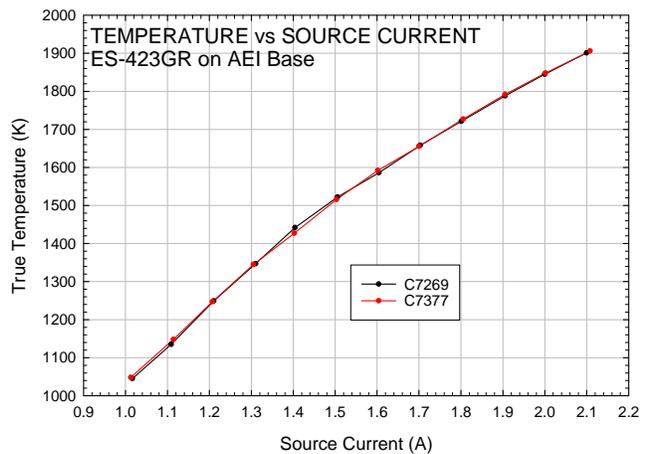
Fig. 2 Typical Operating Parameters of the ES-423GR LaB<sub>6</sub> Cathode
