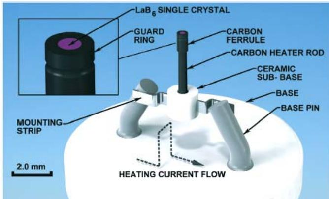
Fig. 1 ES-423GR Guard Ring LaB<sub>6</sub> Single Crystal Cathode on AEI Base
