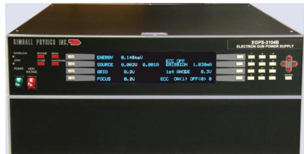
*EGPS-3104B Electron Gun Power Supply with FlexPanel controller*
