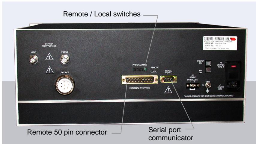
**Fig. 4.4-1 A typical power supply rear panel with 50 pin EXTERNAL INTERFACE connector and RS-232 serial port for remote control and metering of included power supplies (Gun connectors and details will vary with the supply model).**
