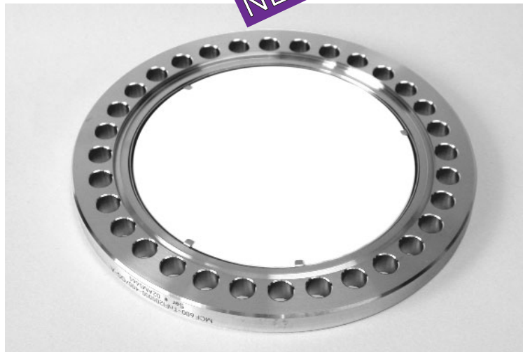
UHV Phosphor Screen on conductive glass, mounted in a 6 inch CF double-sided Thin Flange The Thin Flange is 0.4" thick and must be sandwiched between a window flange and the corresponding system CF flange.
