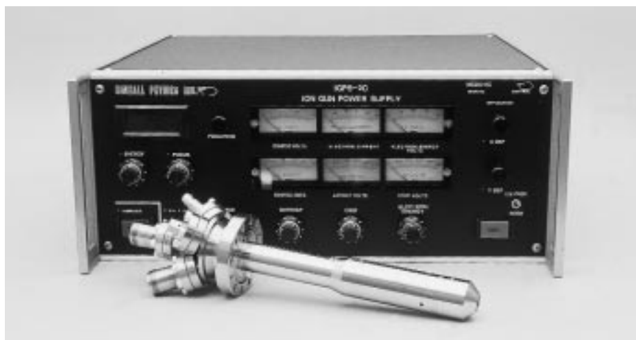
Kimball Physics Ion Gun Power Supply, shown with Ion Gun This system includes the following supplies: Ion Energy, Source with ECC feedback control, Electron Energy, Extract, Grid, Focus, X Deflection, and Y Deflection (Manual controls are on the front panel and remote control terminals on the rear panel)
