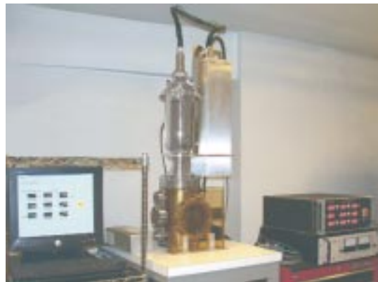
A typical lab set-up of a complete Kimball Physics high energy system with an flood-style electron gun, power supplies and optional computer control system (details vary with gun model)
